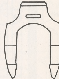
31-7 STEEL CLIP Regularly furnished with all clip mounted locks in place of hex. nut.
