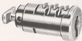
NO. 1769-2-5A Plug retained by a spring actuated crescent. This has a "T" shaped extension which goes through a slot in a panel and when rotated 90° locks across the slot.
