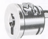
NO. 1734-1 Plug retained by a spring actuated brass crescent. Eccentric pin on rear of plug actuates locking device. Due to shortness this plug is equipped with 3 tumblers.
