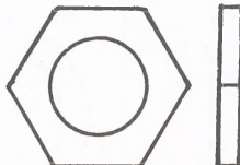
NO. 3186-12 HEX. NUT \frac{5}{32} " thick x \frac{1}{2} "—20 thread steel hex. nut.
